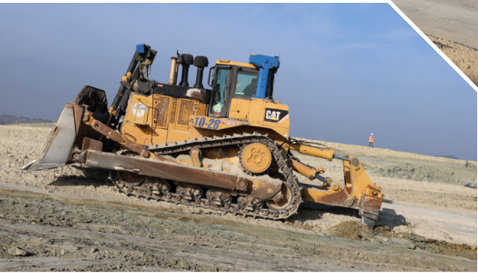
Above Left: One of Coburn Equipment Rentals' operated Cat D10 dozers ripping the cut.
